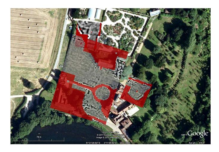
Figure 7. Overlay of geophysical survey results onto Google Earth
