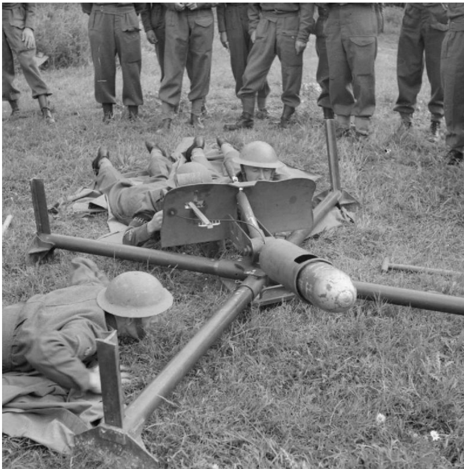
Men of the Saxmundham Home Guard prepare to fire a Blacker Bombard during training with War Office instructors, 30 July 1941. © IWM (H12299)
