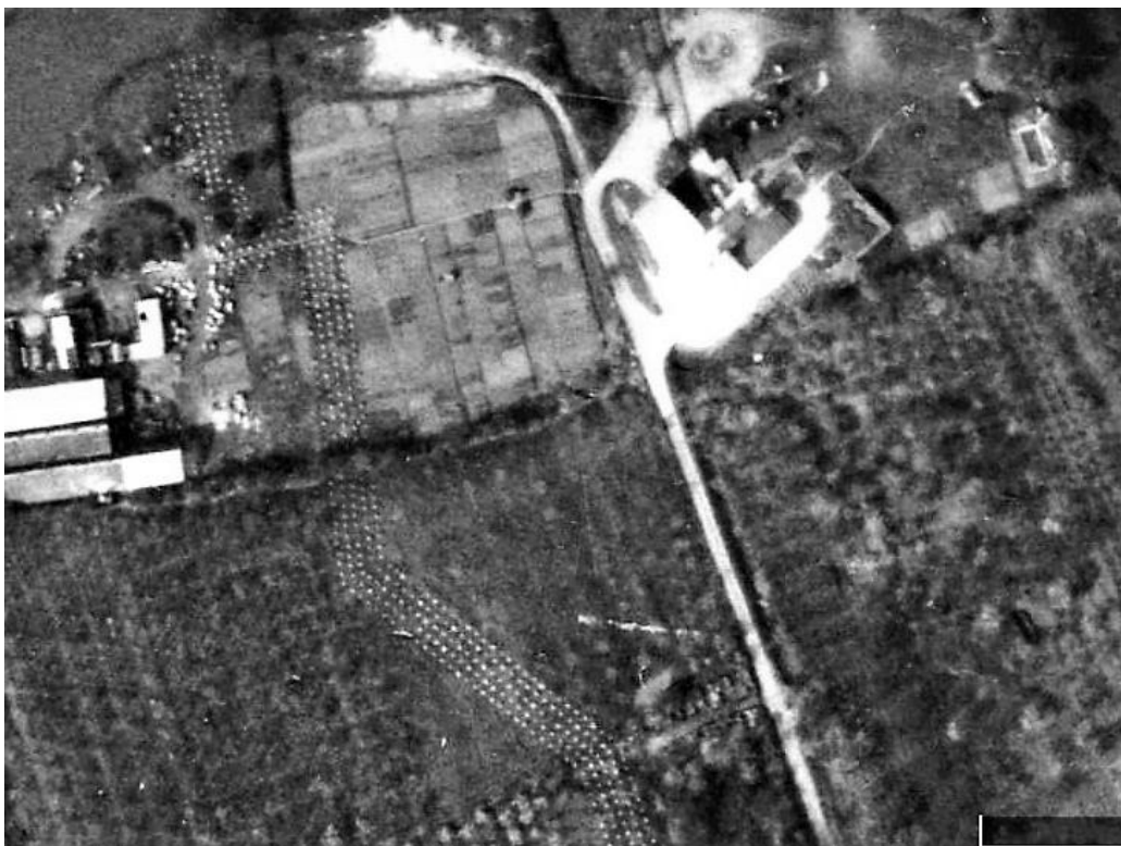
An impressive line of A-T obstacles running along open ground to the banks of the River Medway at Tovil
